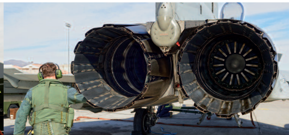
EJ200s – steadfastly delivering 40,000lb thrust
