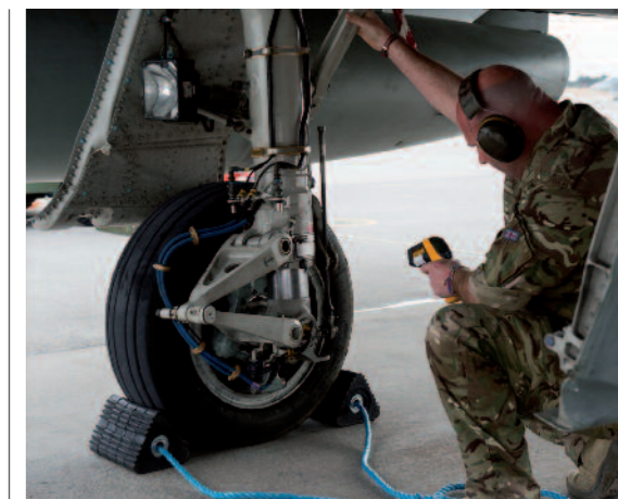
▲ Testing brake temperatures... A vital part of 'post-flight' procedure
