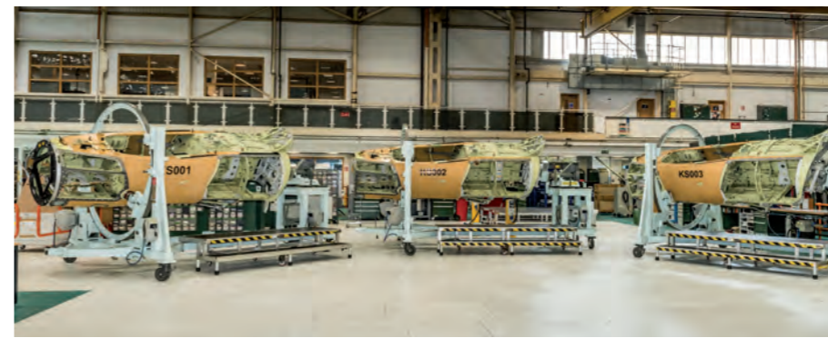
Above: Kuwait front fuselages in assembly at BAE Systems, United Kingdom Below: Eurofighter and Leonardo Kuwait Team
